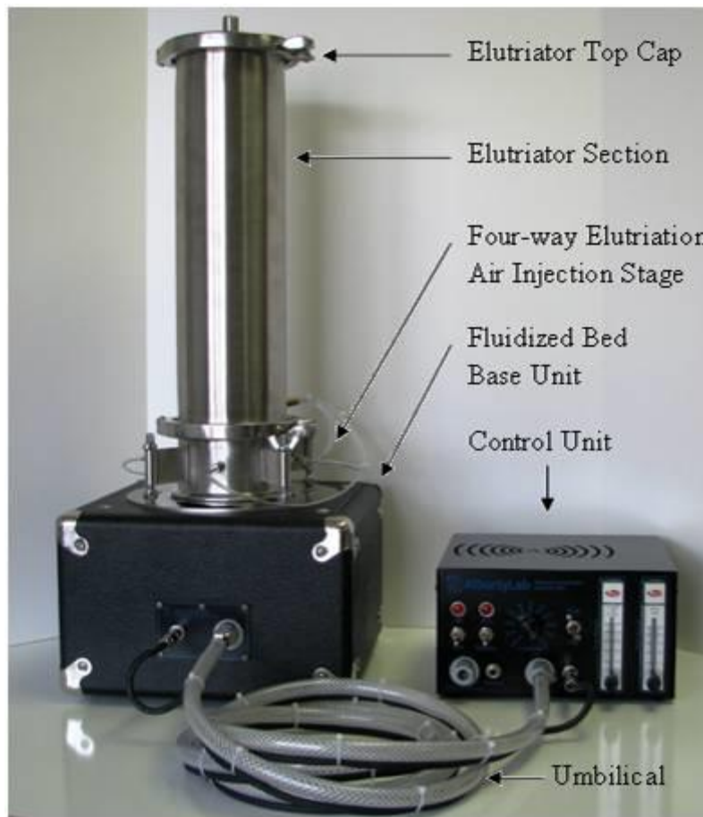
Figure 2. Primary Components of the AG-5025
